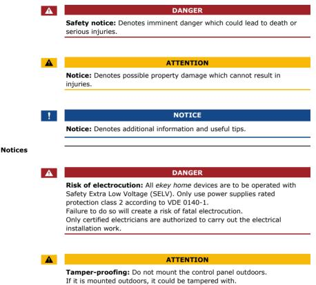
Mount the control panel in a secure internal area.
