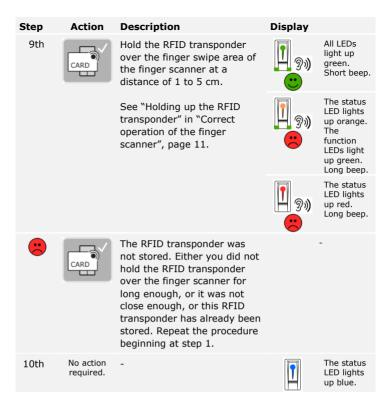
The RFID transponder is stored. The system is in normal mode.
