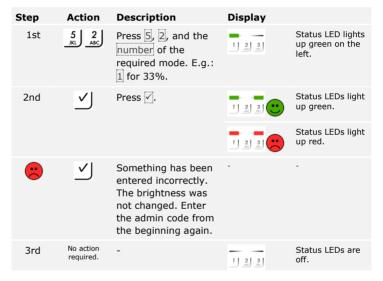
The back-illumination brightness was set. The system is in normal mode.
