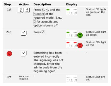
The optical and acoustic signaling to indicate that a button has been pressed was set. The system is in normal mode.
