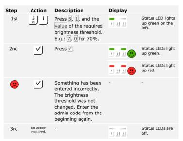
The automatic back-illumination was set. The system is in normal mode.
