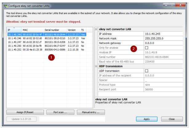
Fig. 20: CONFIGURE EKEY NET CONVERTER LANS: Areas
